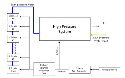
humidistat (0-10V) controls the solenoids controlled card (for proportional working mode) as well as the activation (threshold set at 1V) of the high pressure system.
