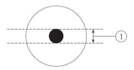
If oil level is not within ① zone, add or remove oil in the tank. Check for oil leaks.
