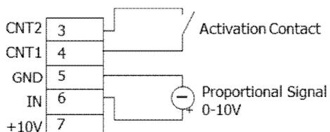
Connect the proportional external regulator outputs between GND and IN terminals as shown in the diagram.
