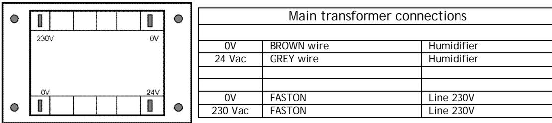
Connect power line to the transformer.
