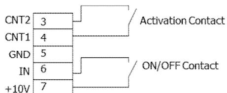
Connect the outputs of the external regulator ON/OFF or humidistat between terminals IN and + 10V as shown in the diagram.
