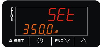
Fig. 4. First start-up - Setting the electrical conductivity
