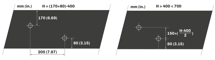
Fig. 36. Horizontal installation - 2 distributors
