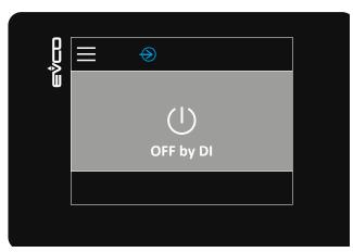
Fig. 17. Humidifier OFF (by digital input)
