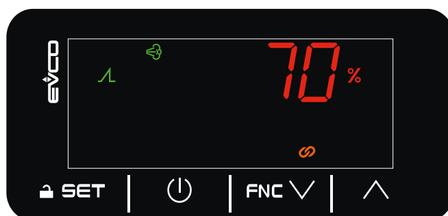
Fig. 38. Home screen with proportional regulation (CFG = PROP)
