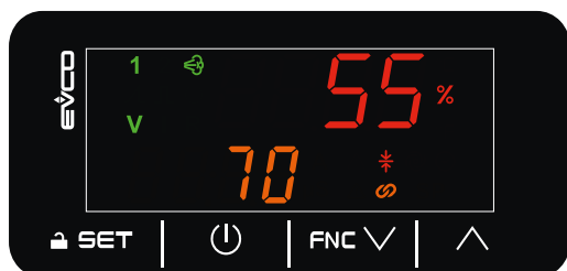
Fig. 39. Home screen with humidity sensor alone
