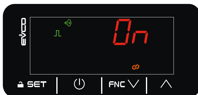
Fig. 37. Home screen with ON/OFF regulation from digital input (CFG = 0-1)
