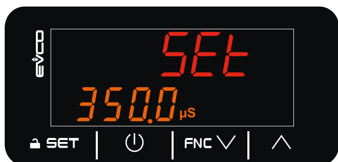
Fig. 35. First start-up - Setting the electrical conductivity
