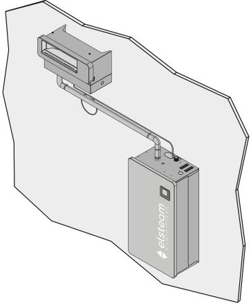
Fig. 39. Remote ventilated steam distribution
