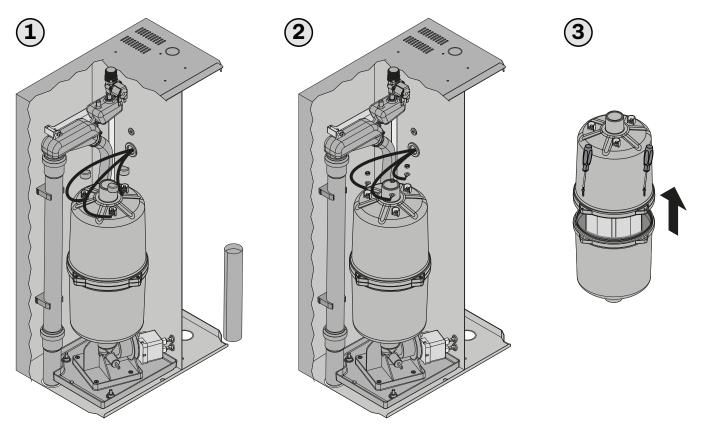
Fig. 115. Replacing the boiler
