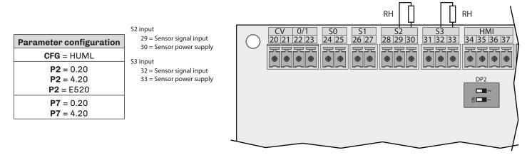
Fig. 100. Connection for humidity sensor and limit sensor (CFG = HUML)
