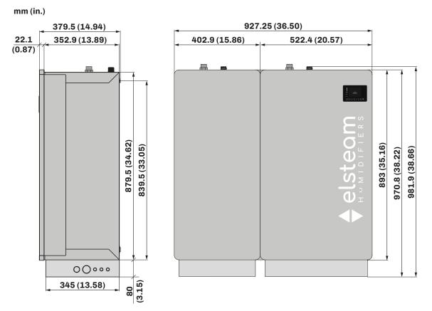
Fig. 28. Dimensions of double boiler models
