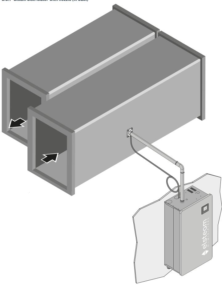
Fig. 44. Steam distributor with nozzle (in duct)
