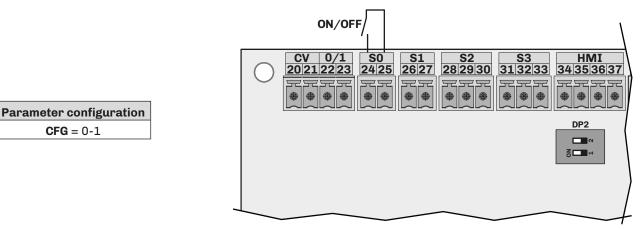
Fig. 57. ON/OFF connection with humidistat or external contact (CFG = 0-1)
