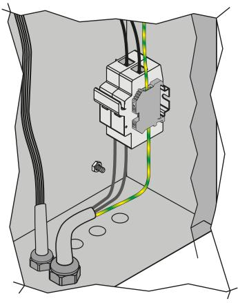
Fig. 104. Power supply connections - single-phase models
