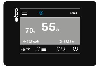
Fig. 20. Home screen with humidity sensor alone
