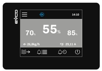
Fig. 21. Home screen with humidity sensor and limit sensor
