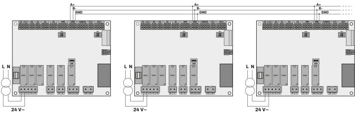
EXAMPLE OF RS-485 CONNECTION WITH SEPARATE POWER SUPPLIES
