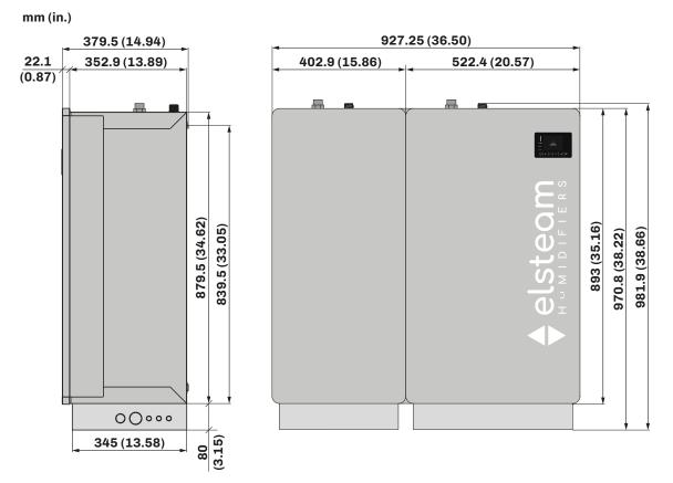
Fig. 81. Dimensions of double boiler models
