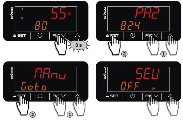
Fig. 74. Output functional test
