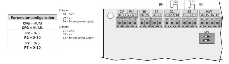
Fig. 103. Humidity sensor connection 0...5 V
