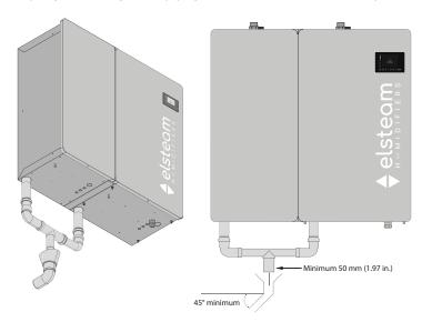
Fig. 34. Specifications of drain pipe for double boiler models - single drain
