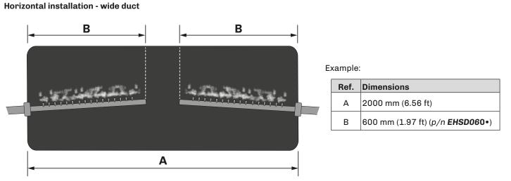
Fig. 38. Horizontal installation in a wide duct - 2 distributors
