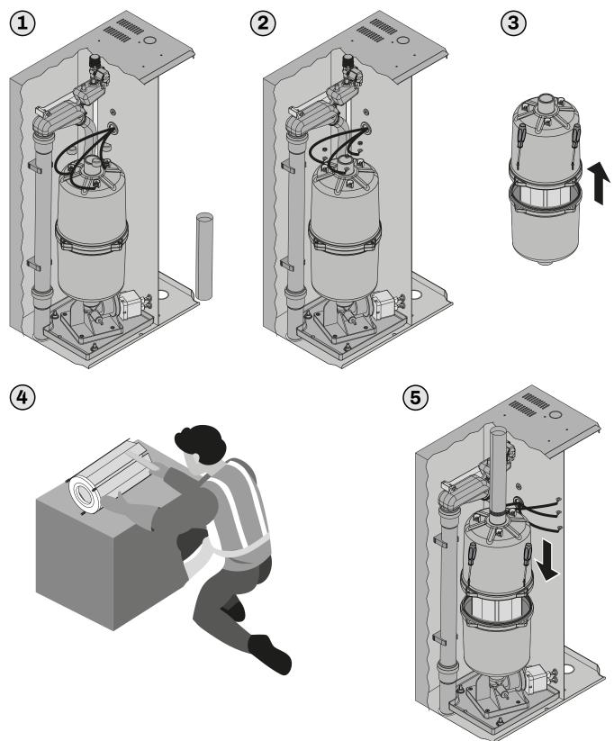
Fig. 116. Cleaning/replacing the electrodes
