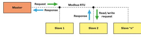
Fig. 70. Diagram showing message exchange in a Modbus communication
