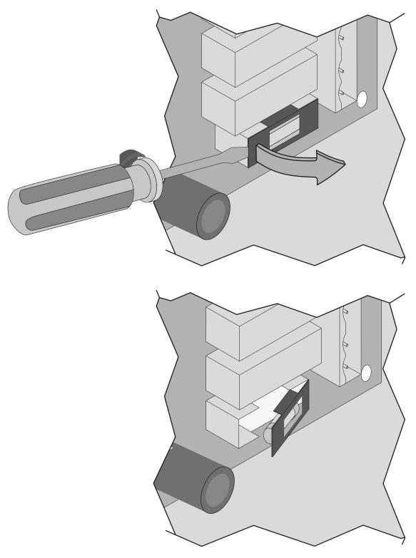
Fig. 54. Protection devices on the control board
