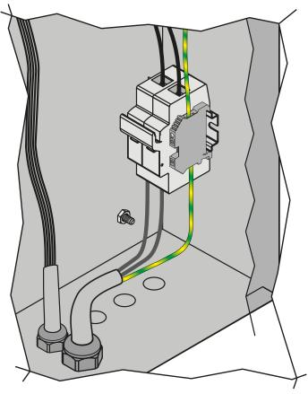
Fig. 65. Power supply connections - single-phase models
