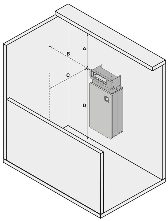
Fig. 42. Minimum distances with installation above the humidifier
