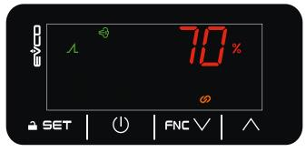
**Fig. 7.** Home screen with proportional regulation (**CFG** = PROP)
