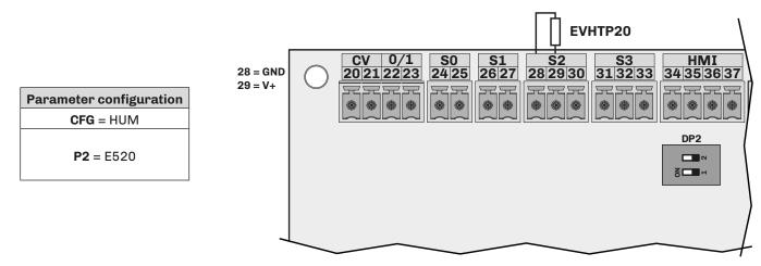
Fig. 60. Humidity sensor connection EVHTP520 (CFG = HUM)
