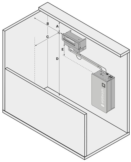
Fig. 41. Minimum distances with remote installation
