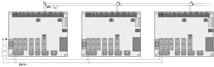
Fig. 69. Serial line connections
