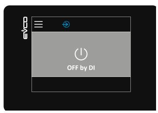
Fig. 17. Humidifier OFF (by digital input)
