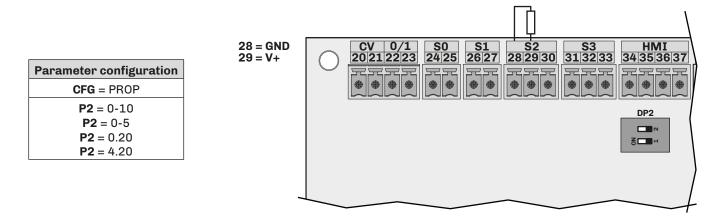
Fig. 97. External proportional humidistat connection (CFG = PROP)
