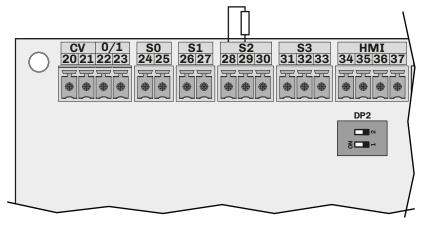
Fig. 62. Temperature sensor connection (CFG = 1T)
