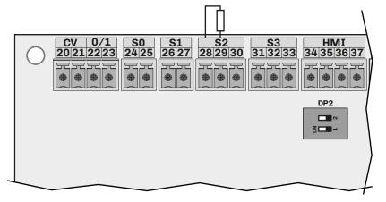
Fig. 101. Temperature sensor connection (CFG = 1T)
