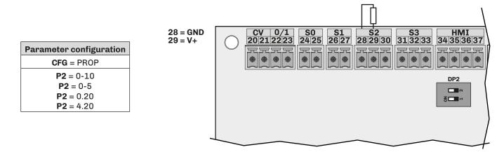
Fig. 58. External proportional humidistat connection (CFG = PROP)
