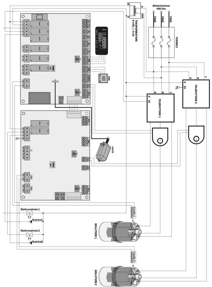
Fig. 123. Wiring diagram models EHKT060T4
