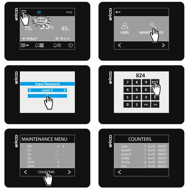
Fig. 76. Displaying the operating hours
