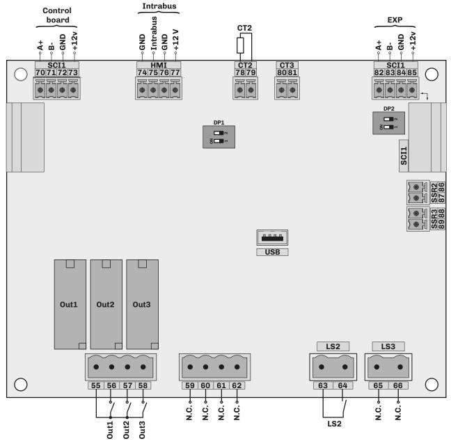
Fig. 95. Expansion electrical connections
