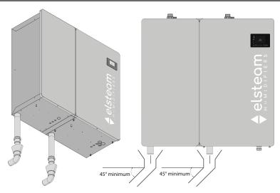
Fig. 33. Specifications of drain pipe for double boiler models - separate drains
