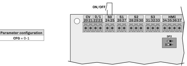
Fig. 96. ON/OFF connection with humidistat or external contact (CFG = 0-1)
