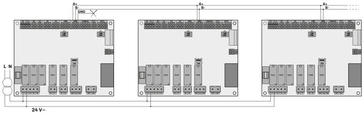
Fig. 108. Serial line connections
