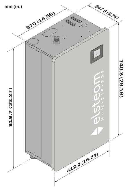
Fig. 78. Dimensions of models EHK•003 ... EHK•015
