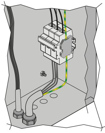
Fig. 105. Power supply connections - three-phase models
