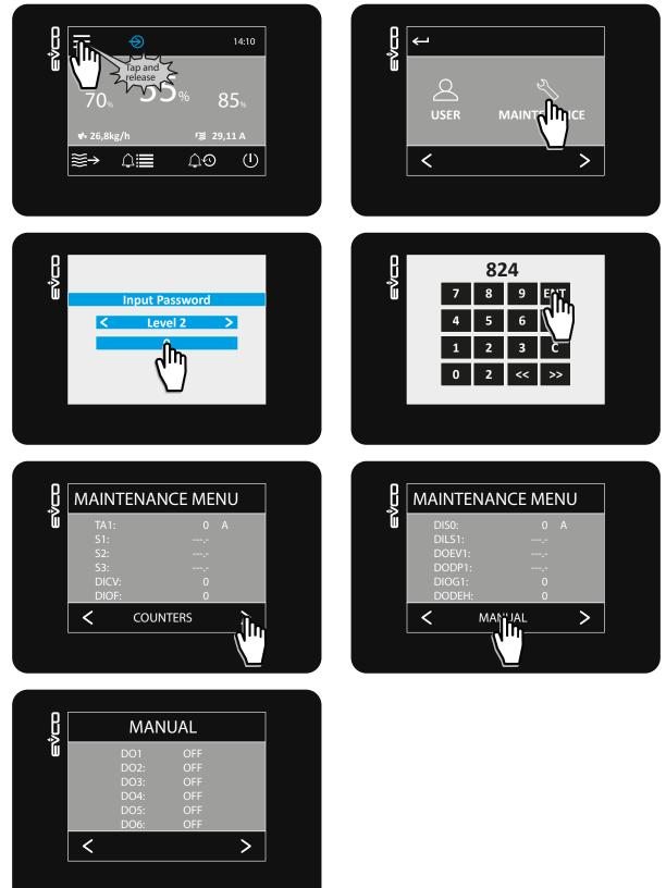
Fig. 77. Displaying the operating hours
