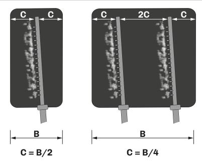
Fig. 37. Vertical installation - 1–2 distributors
