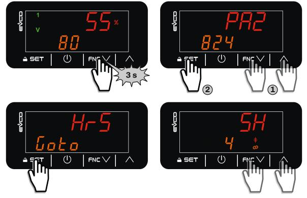
Fig. 73. Displaying the operating hours
