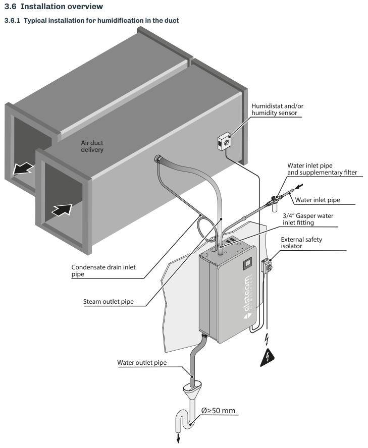
Fig. 45. Typical installation for humidification in the duct
