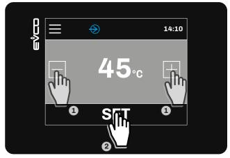
Fig. 23. Changing the temperature setpoint
