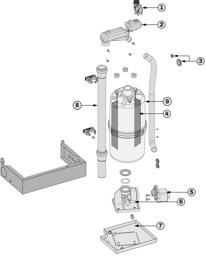
Fig. 117. EHKT/EHKX series spare parts - Plumbing Part
