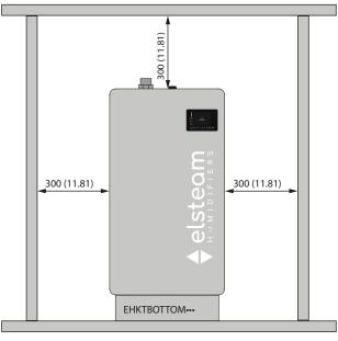
Fig. 82. Minimum installation distances
