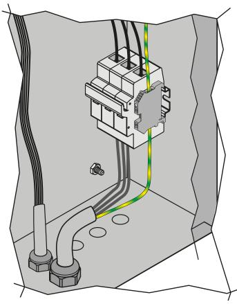
Fig. 66. Power supply connections - three-phase models
