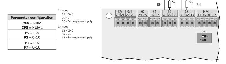
Fig. 64. Humidity sensor connection 0...5 V
