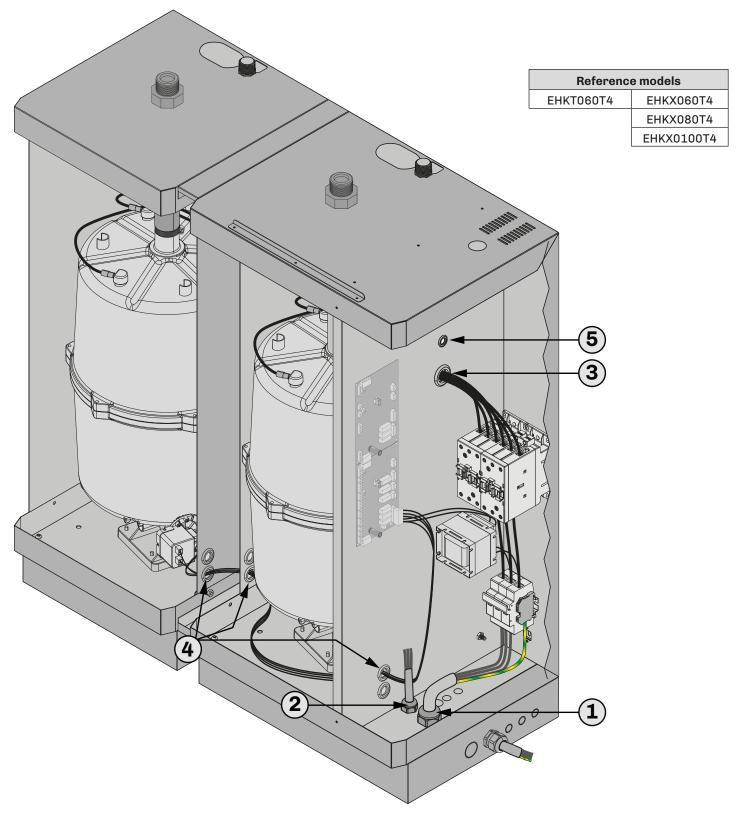
Fig. 107. Cable glands and cable routing
