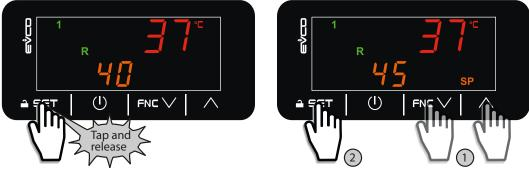
Fig. 11. Changing the temperature setpoint
