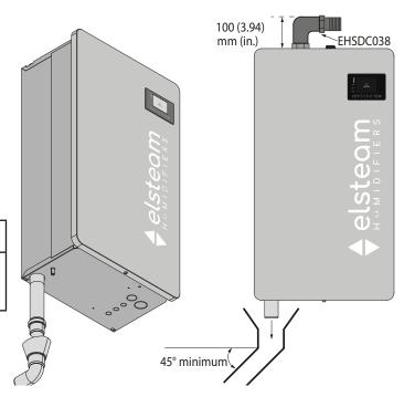
Fig. 32. Specifications of drain pipe for single boiler models
