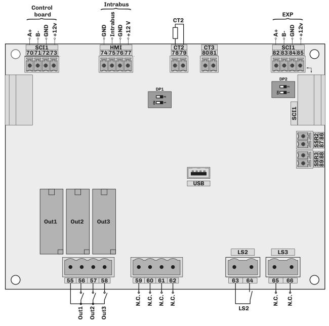
Fig. 56. Expansion electrical connections
