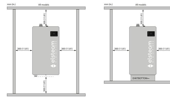
Fig. 29. Minimum installation distances
