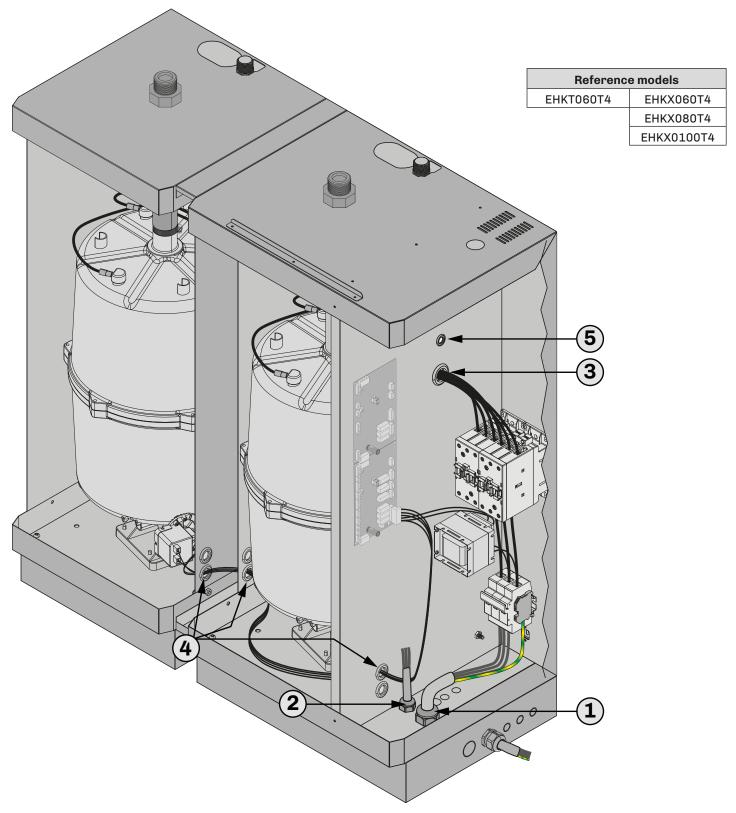
Fig. 68. Cable glands and cable routing
