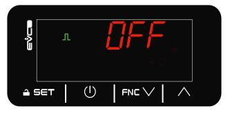
Fig. 27. ON/OFF operation - ID1 and ID2 open
