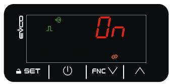
**Fig. 34.** Home screen with ON/OFF regulation from digital input (CFG = 0-1)
