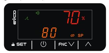
Fig. 35. Home screen with proportional regulation (CFG = PROP)
