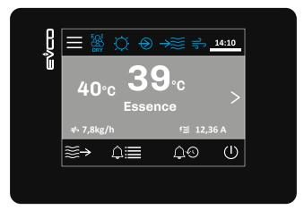
Fig. 43. HOME screen with ON/OFF regulation from digital input - EHKXinterface
