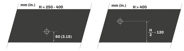
Fig. 13. Horizontal installation - 1 distributor
