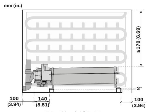
Fig. 7. Minimum installation distances
