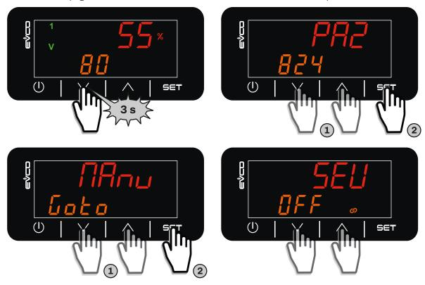
Fig. 45. Output functional test
