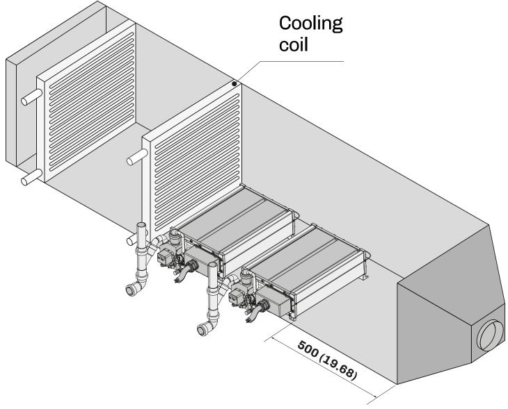
Fig. 9. Minimum installation distances from the droplet separator for two hydraulic units
