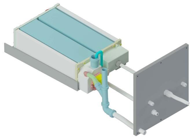
Fig. 2. Hydraulic unit extraction flange
