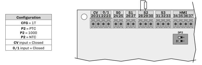
Fig. 28. Temperature sensor connection (CFG = 1T)
