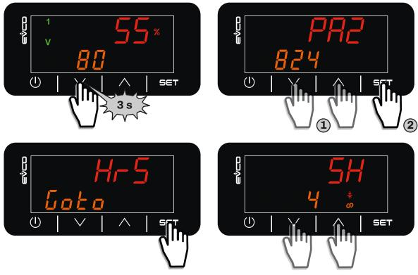
Fig. 44. Displaying the operating hours
