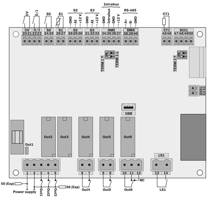
Fig. 21. Control board electrical connections
