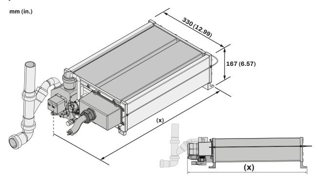
Fig. 5. Hydraulic unit dimensions
