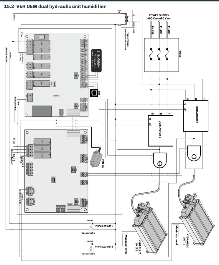
Fig. 54. Wiring diagram for dual hydraulic unit humidifier
