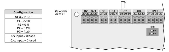
Fig. 24. External proportional humidistat connection (CFG = PROP)
