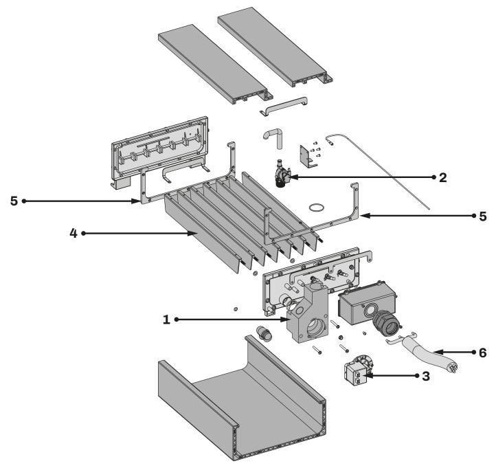
Fig. 51. Spare parts for VEH OEM - Hydraulic unit
