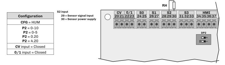
**Fig. 25.** Humidity sensor connection (**CFG** = HUM)
