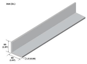
Fig. 4. Corner bracket dimensions
