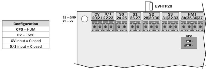
Fig. 26. Humidity sensor connection EVHTP520 (CFG = HUM)
