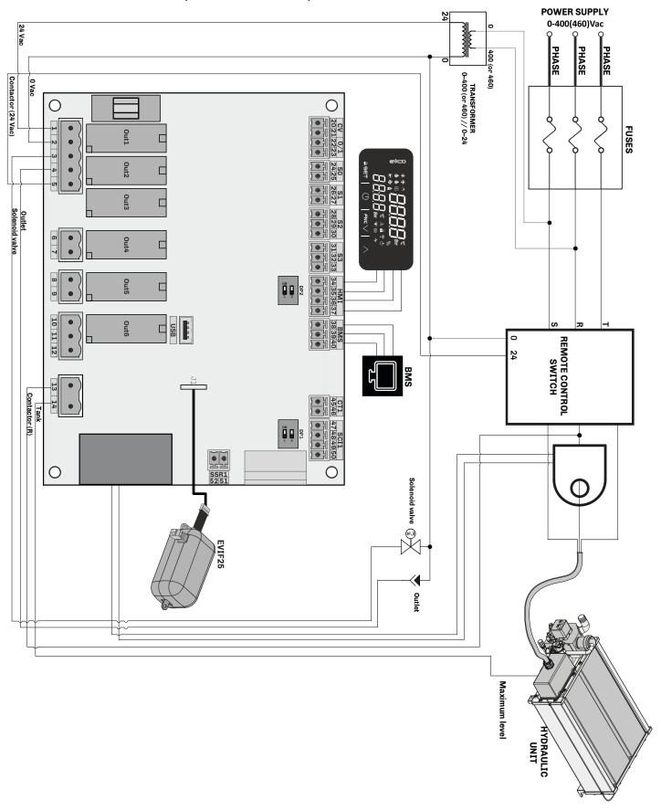
Fig. 53. Wiring diagram for 4- or 7-electrode models
