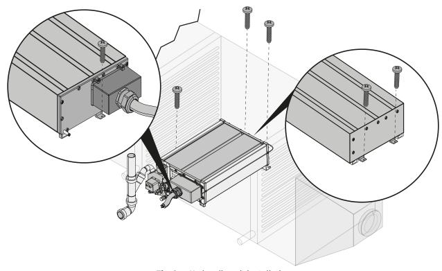
Fig. 6. Hydraulic unit installation
