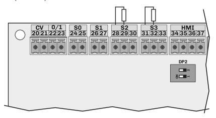
Fig. 29. Temperature sensor connection (CFG = 2T)
