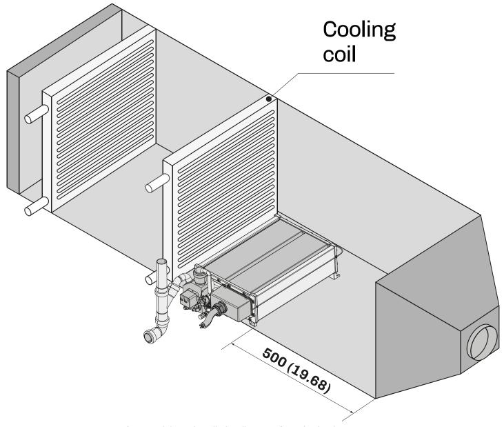
Fig. 8. Minimum installation distances from the droplet separator
