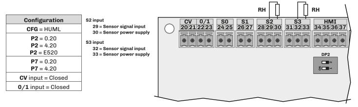
Fig. 27. Connection for humidity sensor and limit sensor (CFG = HUML)
