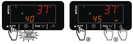
Fig. 39. Changing the temperature setpoint
