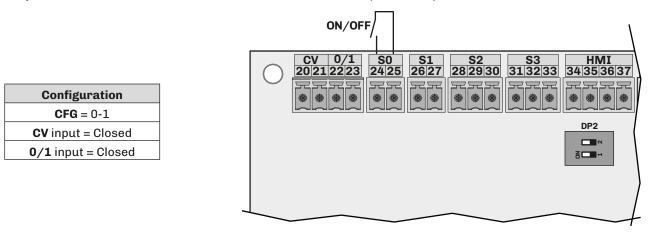
Fig. 23. ON/OFF connection with humidistat or external contact (CFG = 0-1)
