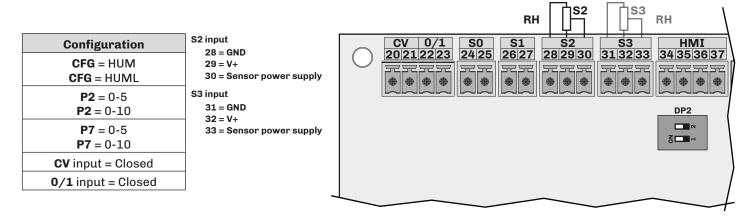
Fig. 30. Humidity sensor connection 0...5 V
